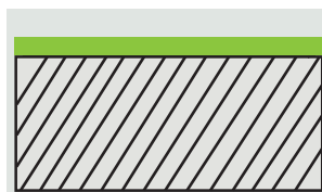
2. Indicator layer Apply RILUMINATI 815 evenly and thinly
