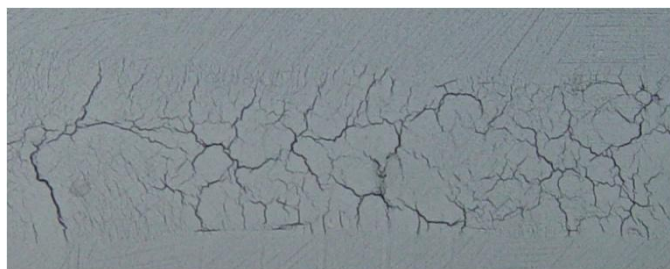
Fig. right: Indications on a welding seam, tested according to EN ISO 9934
